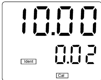
8 Insert the 0.02 NTU calibration standard in the cell shaft
