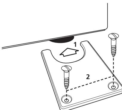
Ensure the unit is positioned correctly. From the sides of the unit, slide the feet brackets around each of the rear feet (1). Secure in place by fixing with two No.8 x 20mm screws (2).
