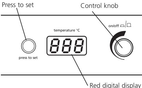
heat to the set temperature. The actual temperature inside the unit will be displayed on the screen. The minimum set temperature is ambient +5°C and the maximum, 60°C.
