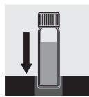
Insert the cell in the photometer cell shaft and start measurement.
