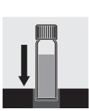
Insert the cell in the photometer cell shaft and start measurement.
