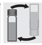
Mix the contents by carefully swaying the cell (10 x).
