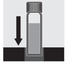
Insert the cell in the photometer cell shaft and start measurement.
