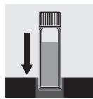
**Carefully** insert the cell in the photometer cell shaft and start measurement.
