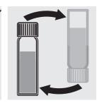
Mix the contents by carefully swaying the cell (10 x). Undissolved powder has no adverse effect on
