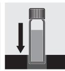
photometer cell shaft and start measurement.
