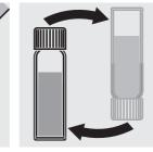
Mix the contents by carefully swaying the cell (10 x). A small amount of solids may remain undissolved.
