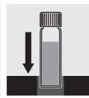
photometer cell shaft and start measurement.
