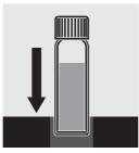
photometer cell shaft and start measurement.
