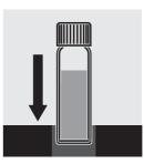
Insert the cell in the photometer cell shaft and start measurement.
