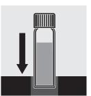
Insert the cell in the photometer cell shaft <u>within one minute</u> and start measurement.
