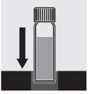
Insert the cell in the photometer cell shaft and start measurement.
