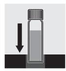
Pipette 5.0 ml of sample Insert the cell in the into a reaction cell, close the cell with the screw cap and mix.
